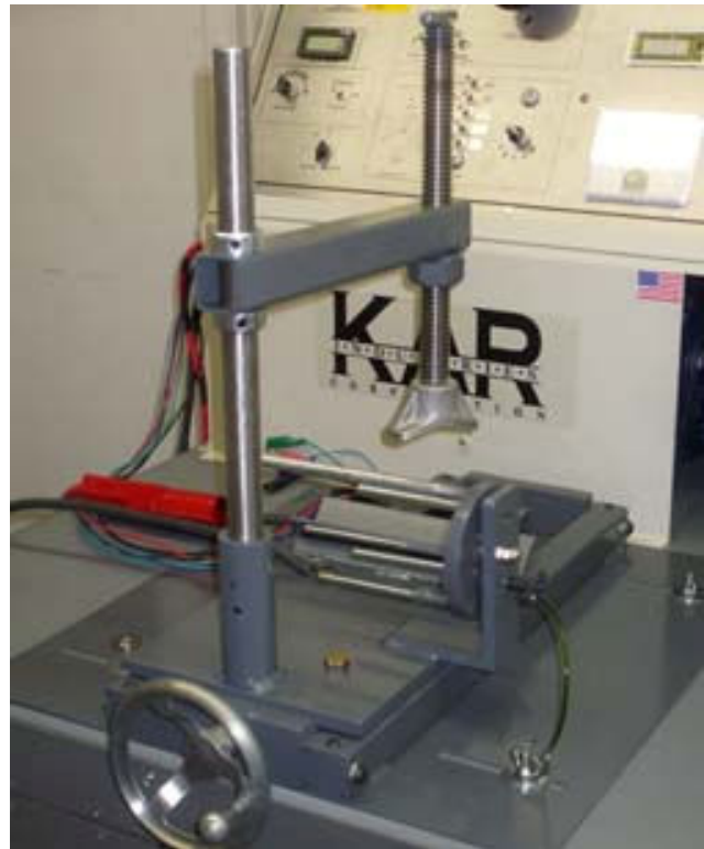
8.- Regular mounting vise with turret for standard alternators
