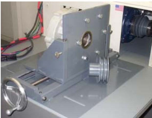
3.- Base, mounting plate and pulley for 50DN 600 series
