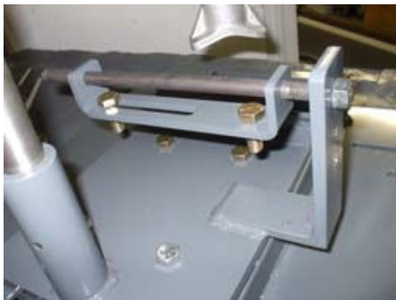
7.-# 6 with bracket to attach to 50DN 500 series.
