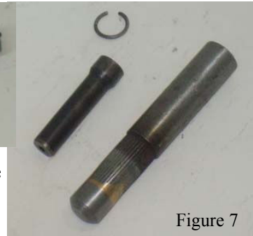
K108-0700-07 Tool to insert the reusable snap ring.
