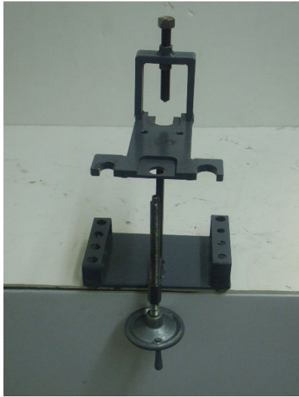
K108-0700-1 Fixture to press drive
